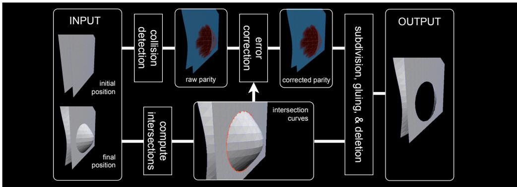
Figure 5: Overview of our method and its components
